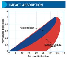
Hysteresis (Mechanical Energy converted to heat each cycle)
